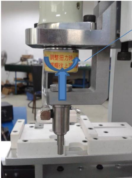
firstly pull up the knob then turn it for torque adjustment.
